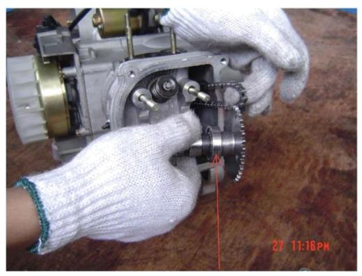
Fig. 8. Install the camshaft.
