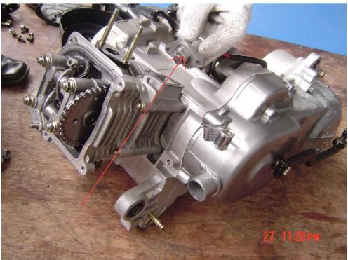
Fig. 12. Install chain tension assembly.
