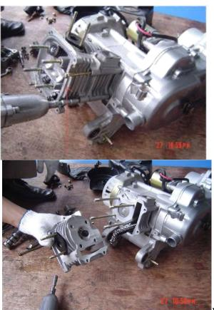
Fig. 11. Remove cylinder head.
