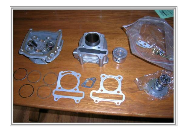
The following is a general guide for installing a big bore kit OR rebuilding the GY6 type engine. The photographs in this booklet are installing an 80cc bore kit in a 50cc GY6. Readers should take not that there can be minor variations in this as there are numerous companies in China who manufacture the GY6.
