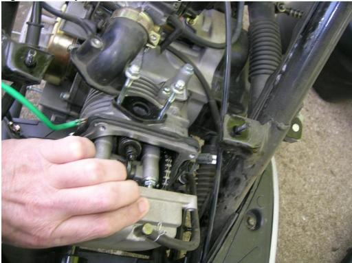
Fig. 5. Remove cylinder head cover.
