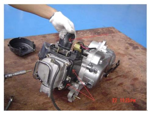
Fig. 16. Install carb inlet tube.
