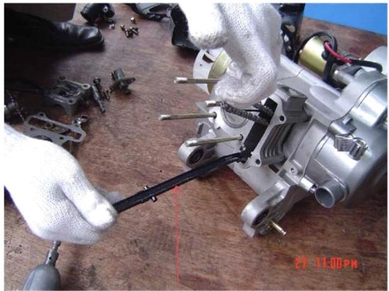
Fig. 13. Remove chain guide.
