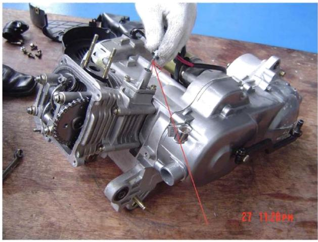
Fig. 12b. Install chain tension.
