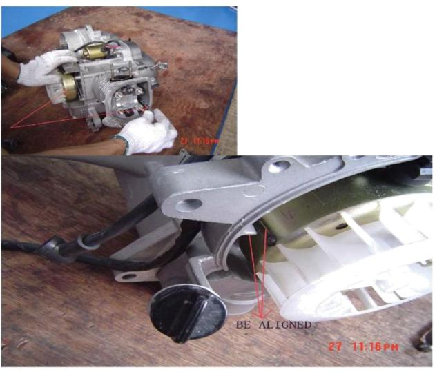
Fig 7. a & b. Install the cylinder head. Rotate the magneto and chain until the markings are lined up.
