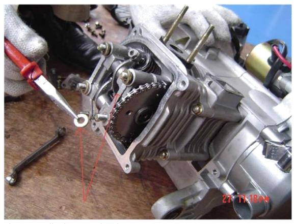
Fig. 11. Install valve seat and washers
