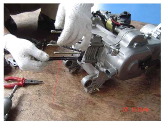
Fig. 5. Install the chain guide.
