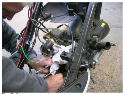
Fig. 17. Protect engine opening.
