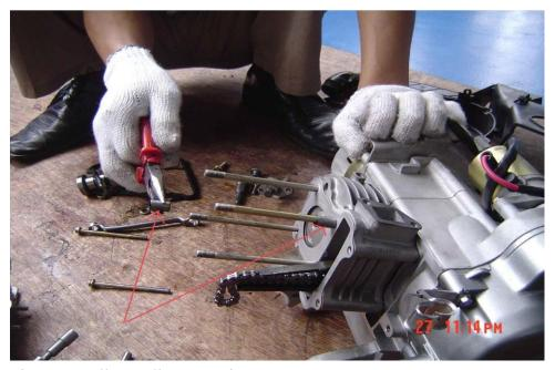
Fig. 6. Install two alignment pins.
