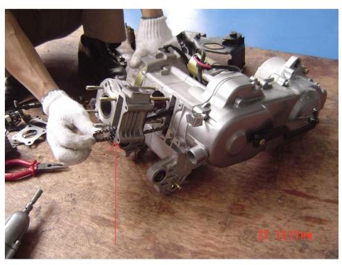
Fig. 4. Install the cylinder over the piston.
