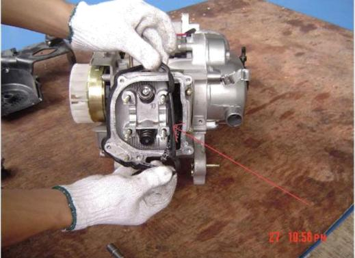
Fig. 10. Remove Gasket.
