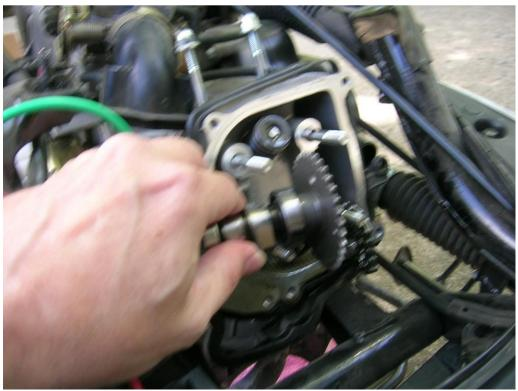
Figs. 9 a & b. Remove the camshaft.
