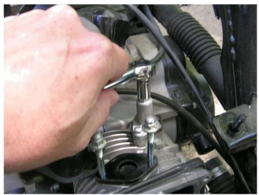
Fig. 8. Remove the chain regulator
