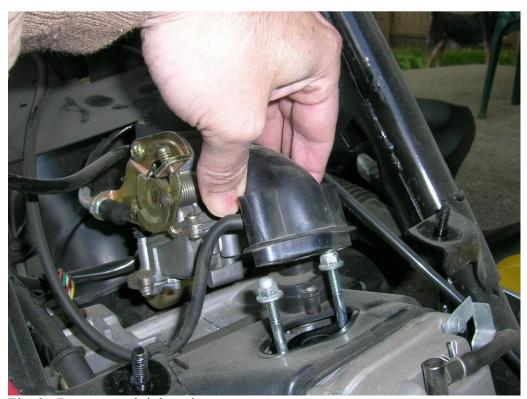
Fig. 3. Remove carb inlet tube.
